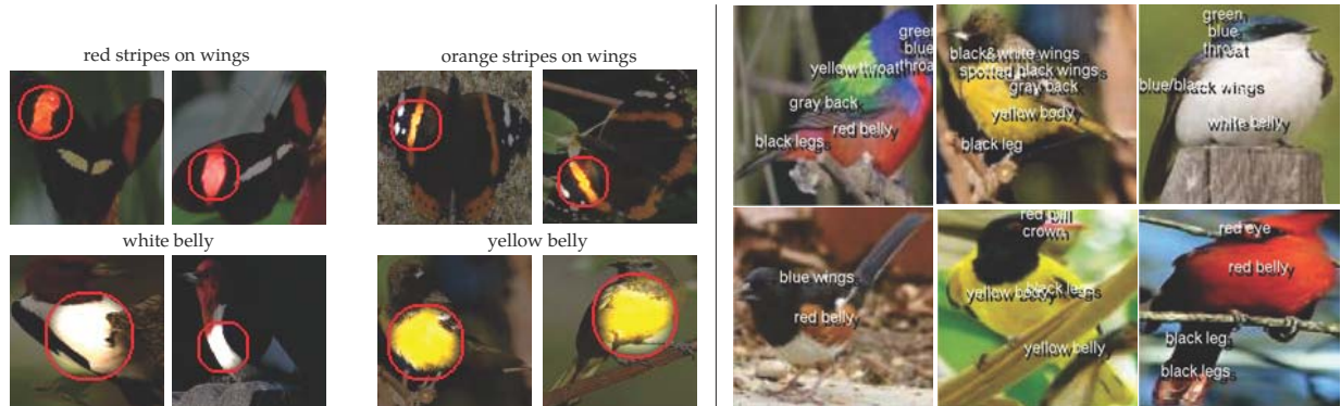
Figure 4: Results of our attribute-based recognition approach [65]. Attributes (which are visually distinctive properties that are also nameable and meaningful to humans) are discovered through automated learning with minimal human interaction (left), and then can be detected automatically in new images (right).
