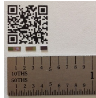
Figure 8: Proposed “peel-and-stick” sensor tag. A 0.5” x 0.5” QR code sits next to our processor (ARM CM-0), radio, and solar cell.
