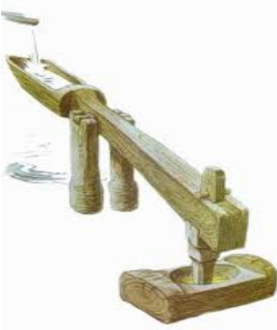
Figure 1: Monjolo (water mill) hammers at a rate that is proportional to the water flow rate.
