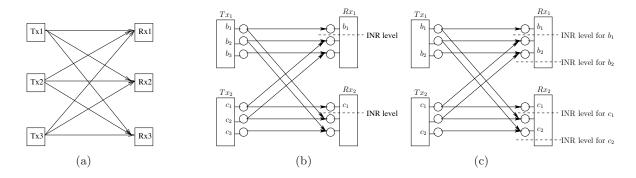
Figure 6: (a) Three user interference channel, (b) achieving sum-rate of 2 by treating interference as noise, and (c) achieving sum-rate of 4 by a more careful assignment of signal levels.
