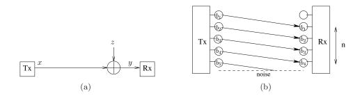
Figure 2: (a) Gaussian model and (b) deterministic model for point-to-point channel.
