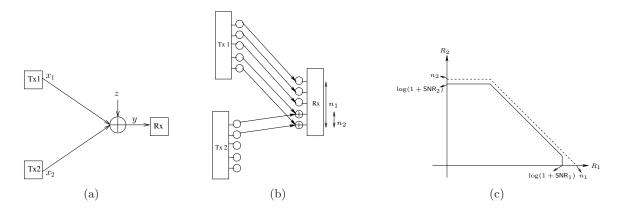
Figure 3: (a) Gaussian model for MAC, (b) deterministic model for MAC, and (c) capacity region of Gaussian MAC (solid) and deterministic MAC (dashed).
